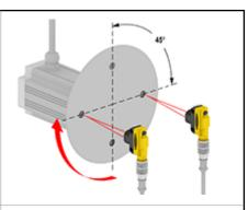
Four sensing points at the same distance from the center of the disk. Each sensor sends **four** pulses per revolution to the Module ( $500 \text{ rpm} = 500 \times 4 = 2,000 \text{ ipm}$ ).
