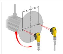
Two sensing points at the same distance from the center of the disk. Each sensor sends **two** pulses per revolution to the Module ( $500 \text{ rpm} = 500 \times 2 = 1,000 \text{ ipm}$ ).
