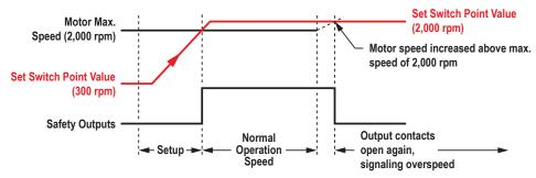
Figure 9. Over-speed Timing
