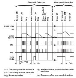
Figure 2. Functional Diagram
