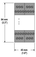
Figure 10. Dimensions—SSM-FM-11A20
