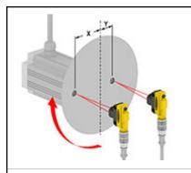
Two sensing points at different distances from the center of the disk. Each sensor sends **one** pulse per revolution to the Module (500 rpm = 500 ipm).
