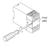
Figure 5. Removing the front cover
