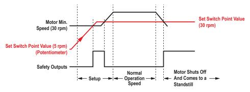
Figure 8. Under-speed Timing
